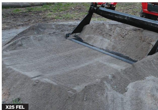
X25 FEL Grab – Position the bucket over material, then close to pick it up.
