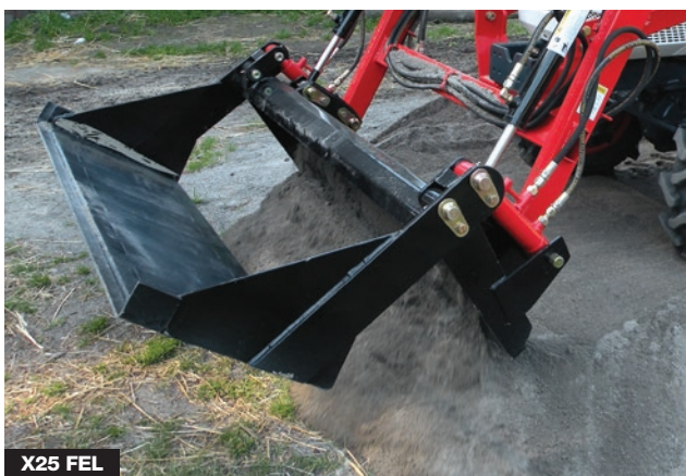
X25 FEL Blade – Bucket open and pushing forward (rear half vertical).
