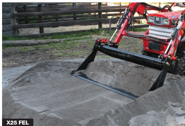
X25 FEL Scrape/Level – Drag bucket backward to scrape or backfill.
