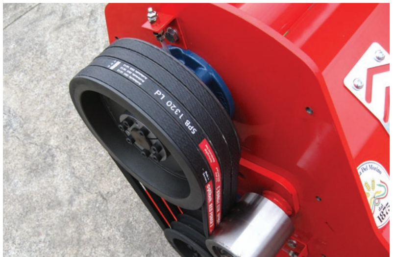
The transmission has four heavy duty belts.
